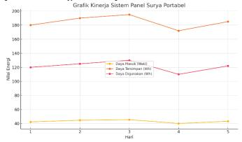
The image above shows a consistent pattern: as the input power increases, the stored power and usable power also increase. Day 3 showed the highest performance, with 45.5W of input power and 96% system efficiency. In contrast, day 4 recorded the lowest input power (40.1W), but the system still provided a fairly high stored and used power, indicating stable system efficiency.
