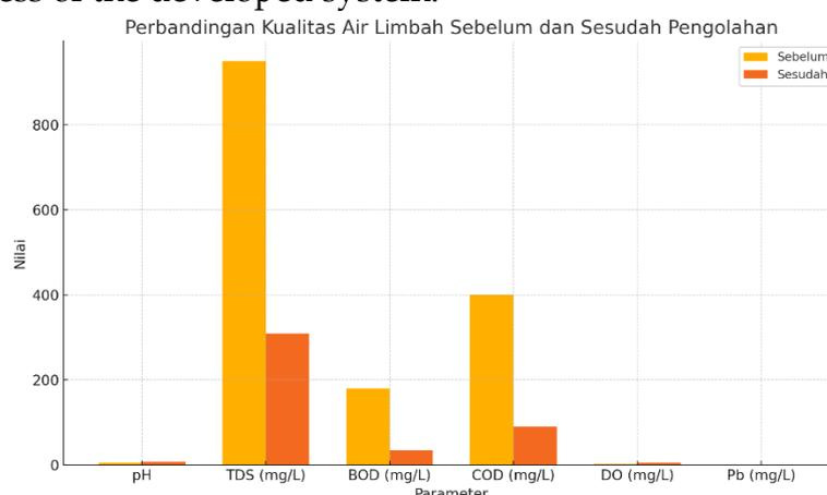
This graph shows that all parameters are changing for the better, with the highest rates of decline occurring in BOD and COD. This signifies that the biofiltration system is highly effective in addressing organic pollutants, while smart sensors provide the convenience of monitoring results directly.
